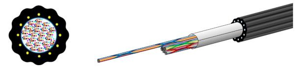
The Wrapping Tube Cable (WTC<sup>™</sup>), with Spider Web Ribbon (SWR<sup>™</sup>), is an ultra-high density outside plant cable designed specifically for fiber-to-the-home (FTTH), access markets, and hyperscale data center. Ultra-high density and a new ribbon technology called Spider Web Ribbon, WTC provides the smallest cable diameter and lowest weight, high-fiber count ribbon cable in the industry. WTC<sup>™</sup> with SWR<sup>™</sup> cables are available in fiber counts from 48 to 864.
