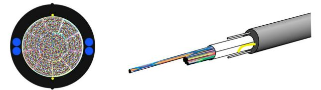
The Wrapping Tube Cable (WTC<sup>™</sup>) with Spider Web Ribbon (SWR<sup>™</sup>) is an ultra-high density outside plant cable designed for fiber-to-the-home (FTTH), access markets, and data centers. It complies with the latest outside plant cable standard, Telcordia GR-20. WTC<sup>™</sup> with SWR<sup>™</sup> offers the smallest cable diameter and lowest weight among high-fiber count ribbon cables in the industry. It is available in fiber counts ranging from 144 to 6,912.
