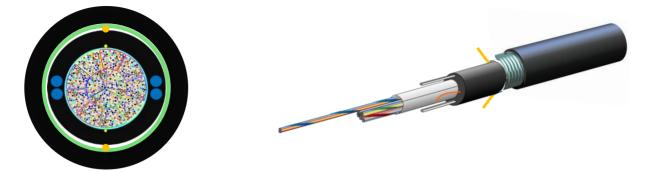
The Wrapping Tube Cable (WTC<sup>™</sup>) with Spider Web Ribbon (SWR<sup>™</sup>) is an ultra-high density outside plant cable designed for fiber-to-the-home (FTTH), access markets, and data centers. It complies with the latest outside plant cable standard, Telcordia GR-20. WTC™ with SWR™ offers the smallest cable diameter and lowest weight among high-fiber count ribbon cables in the industry. It is available in fiber counts ranging from 24 to 864.
