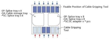
Input/Output Cable Insertion Direction Red: Installation Possible, Blue: Gripping tool is required
