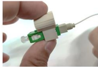
2. Insert the cleaved fiber into the connector
