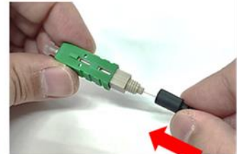
4. Lastly, push the boot onto the connector's body
